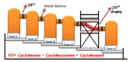
During the late afternoon on 1 June 1974, a 20 inch bypass system ruptured, which may have been caused by a fire, on a nearby 8 inch pipe. This resulted in the escape of a large quantity of cyclohexane. The cyclohexane formed a flammable mixture, and subsequently, found a source of ignition. There was, subsequently, a massive vapour cloud explosion which destroyed the control room where the majority of fatalities occurred, caused extensive damage, and started numerous fires on the site.
